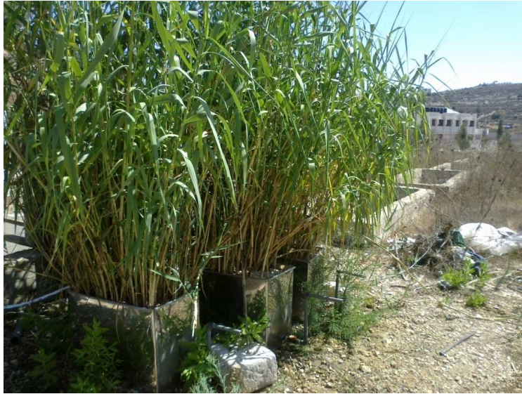
Photo 2 Small scale constructed wetland experimental setup, photo date (27/August/2011)/ Birzeit University/ Palestine
